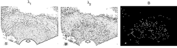
Fig. 3. Image \lambda_1 highlights pixels which are part of elongated structures and image \lambda_2 shows round structures. Image B is a thresholded version of masked I' . Note the granulation in the eigenvalue images is dark because only negative eigenvalues are depicted.
